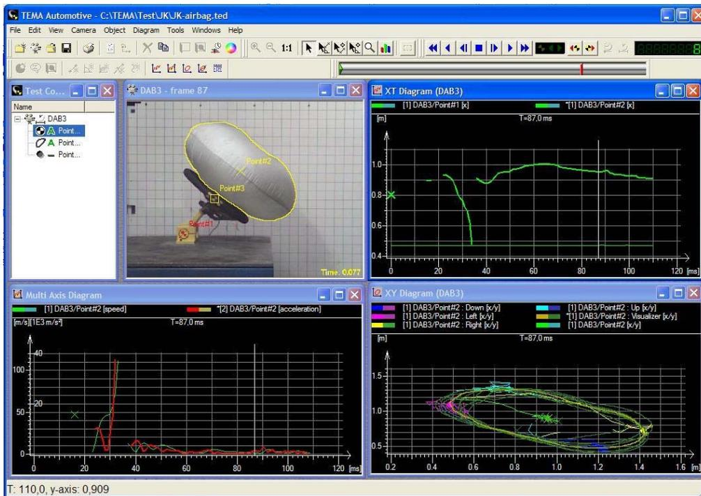
The interface is fully synchronized. Changing a parameter, clicking on an interesting value in a table or moving the time slider to an interesting position on a curve will automatically update all windows and show the corresponding image in the image sequence, curve or table.
