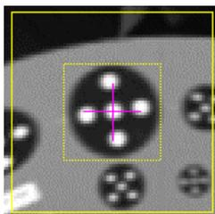
MXT Targets is a special target used in the German Automotive industry. The tracker algorithm finds the symmetry centre of the target.
