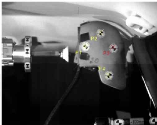
The motion of the rigid body can be described with six parameters: three positions coordinates ( $x$ ,  $y$  and  $z$ ), which gives the position of a specific point on the body, and three attitude angles (roll, pitch and yaw), which gives its orientation in space.
