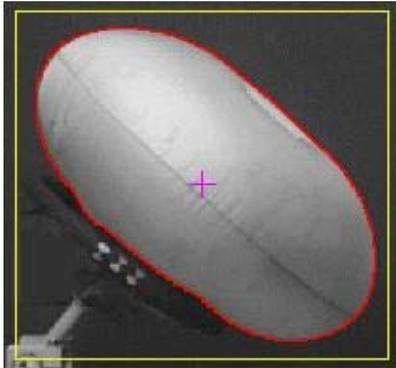
In Airbag contour TEMA searches the object boundary to provide an outline around a body, for instance an airbag.
