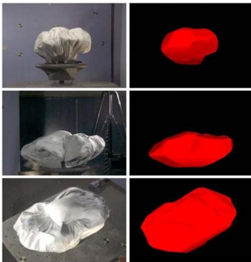
In TEMA Airbag Volume a full 3D model of the airbag is reconstructed from multiple video sequences.
