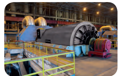
Skoda Power used Optimus to achieve 16% reduction in stress peak values in steam turbine blades. The average stress in sensitive blade regions and the contact pressure between rotating parts also decreased.
